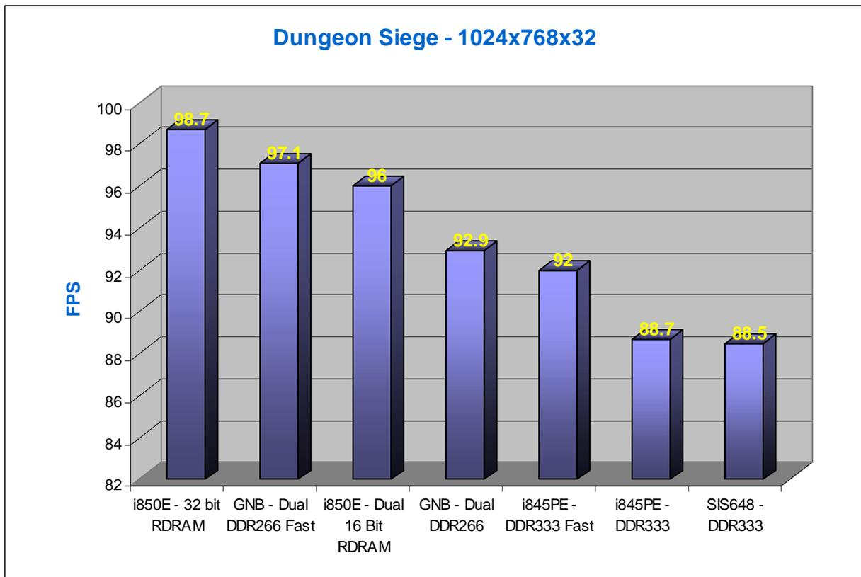
Dungeon siege shows a 4.5% difference between Granite Bay with DDR266 2-2-2-6 and DDR 2-3-3-6, which is quite remarkable. Granite Bay seems to need good quality DDR333 to keep up with the i850E. DDR333 is simply not good enough for the Pentium 4.
