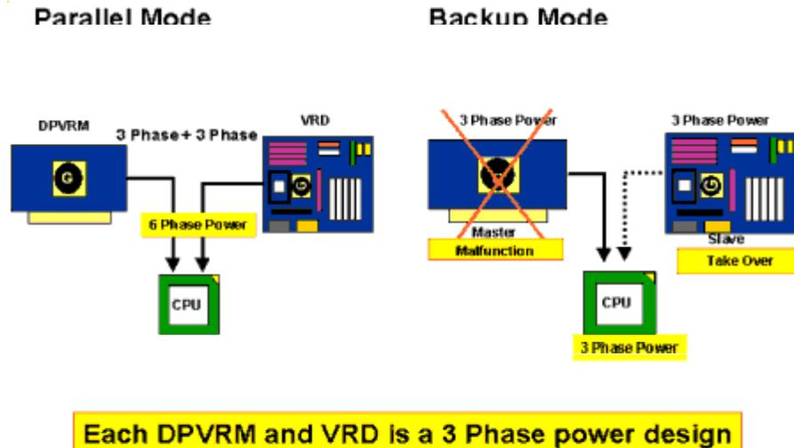
In parallel mode (default) the two 3 phase power regulators should, according to Gigabyte be able to support CPU's up to 10 GHz (up to 150 A!). If one of the VRM fails, the other VRM takes automatically over (backup mode). Gigabyte claims that in parallel mode, the VRMs warm up to 76°C (70 A current) while a single VRM gets 81°C hot.
