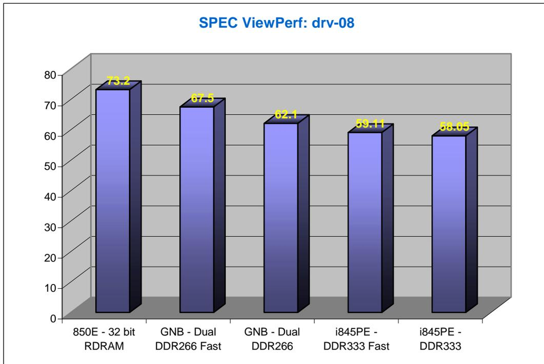
If your workstation is your main tool for designing plants and other complex structures, it is clear that you must invest in the speediest DRAM available. Compared to DDR333, RDRAM is no less than 25 to 31% faster! However, i850E 32 bit RDRAM boards are not an option for this category of software as 1 GB RDRAM are not available. If 2 GB is enough, you can opt for a i850E 16 bit board otherwise a i860 board or a Granite Bay board might be worth considering.
