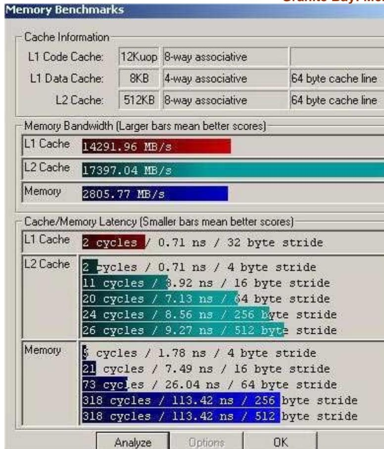
Granite Bay, which has the same theoretical peak bandwidth as the i850E with PC1066, is able to edge the latter out with a few MB/s more. Much lower latency, and slight more bandwidth, that is very promising...
