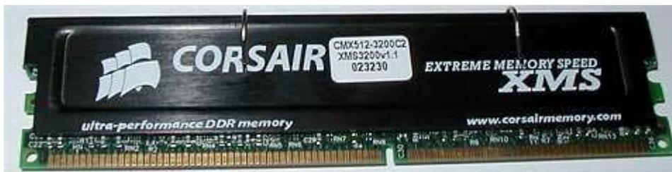
The XMS3000 and XMS3200 we tested are based on 256Mbit Winbond rev B 6ns IC's. The XMS3200 use the best 6ns chips. This might be a bit weird, considering that there are many 5ns IC out there. But most of the current 5ns chips only work at 3-4-4, which is worse than what the 6ns Winbond chips can do. Only the newest Winbond 5ns chips seems to be able to better, and these are the chips that power Corsair's XMS3500
