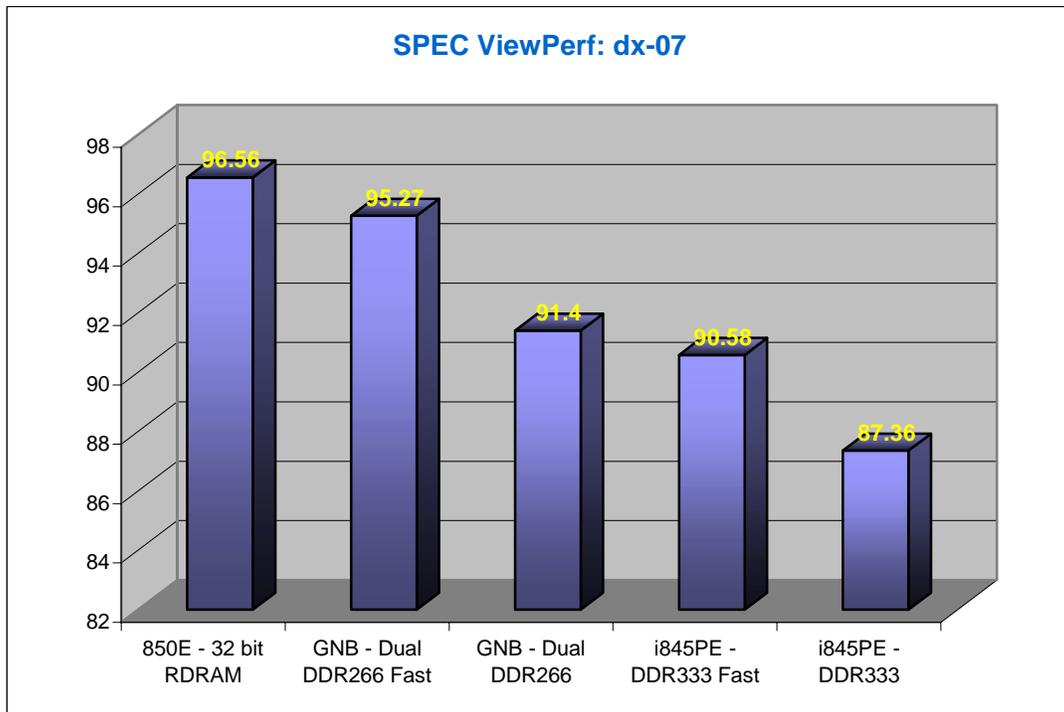
Scientific simulation runs the fastest on the i850E, but the difference with Granite Bay is negligible. Note how the E7205 chipset (GNB) again needs 2-2-2 DDR to shine.
