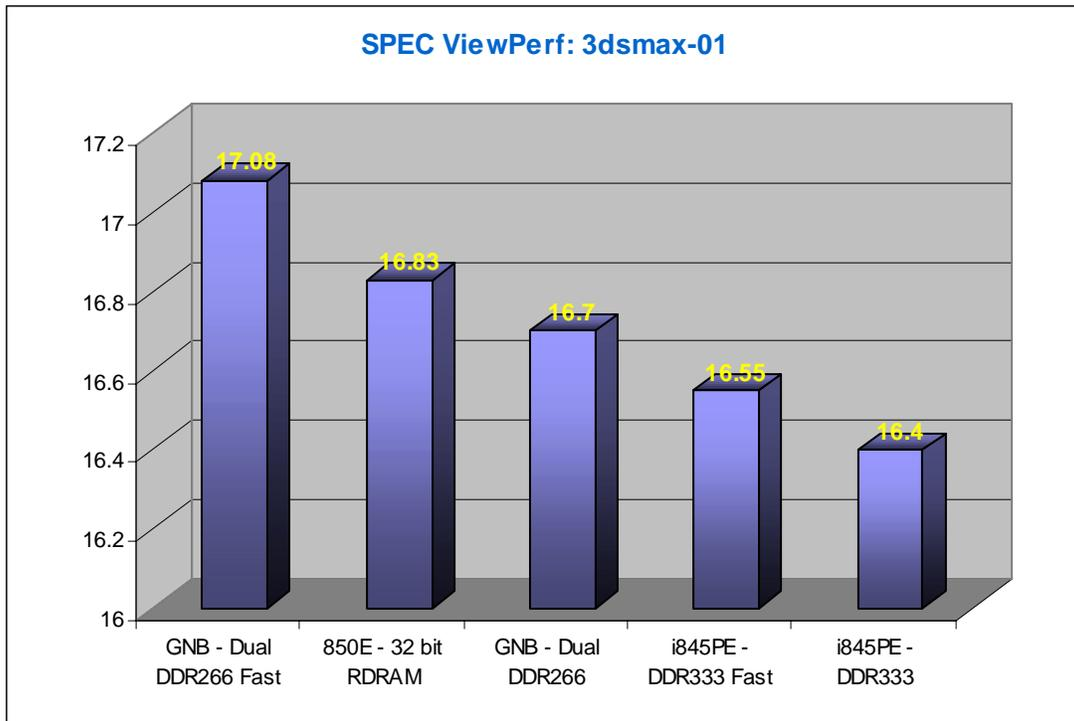
Granite Bay is a tad faster, but needs the boost of the fastest timed DDR266 to pass the i850E. Still, fast DRAM is not that important for 3DSMax modeling, as the fastest chipset is only 3% faster than the cheap i845PE.
