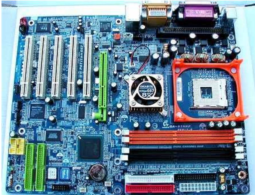
The board also features two RAID controllers: one Silicon Image's 3112A Serial ATA controller which can support two Serial ATA devices in RAID 0 or RAID 1 and one Promise PDC20276 RAID controller which supports the "old" parallel ATA cabled disks. This means you can have up to 10 (!) harddisk with these board! Better get a spacy case...
