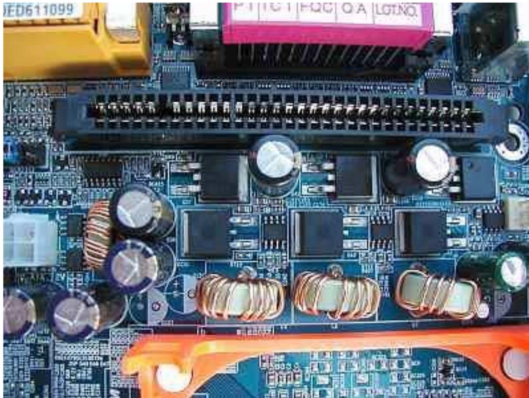
Gigabyte's "Dual Power Voltage Regulator Module" (DPVRM) can work in two modes: parallel and backup mode.
