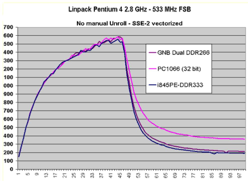
Linpack's results seem very similar to the modify test of PCMark 2002. RDRAM is definitely more efficient here.
