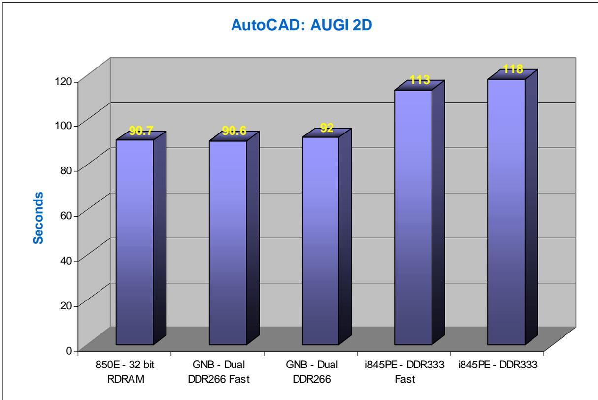
It is remarkable how most workstation applications demand fast memory. DDR333 is a lot slower than the E7205 chipset and all Rambus powered chipsets.
