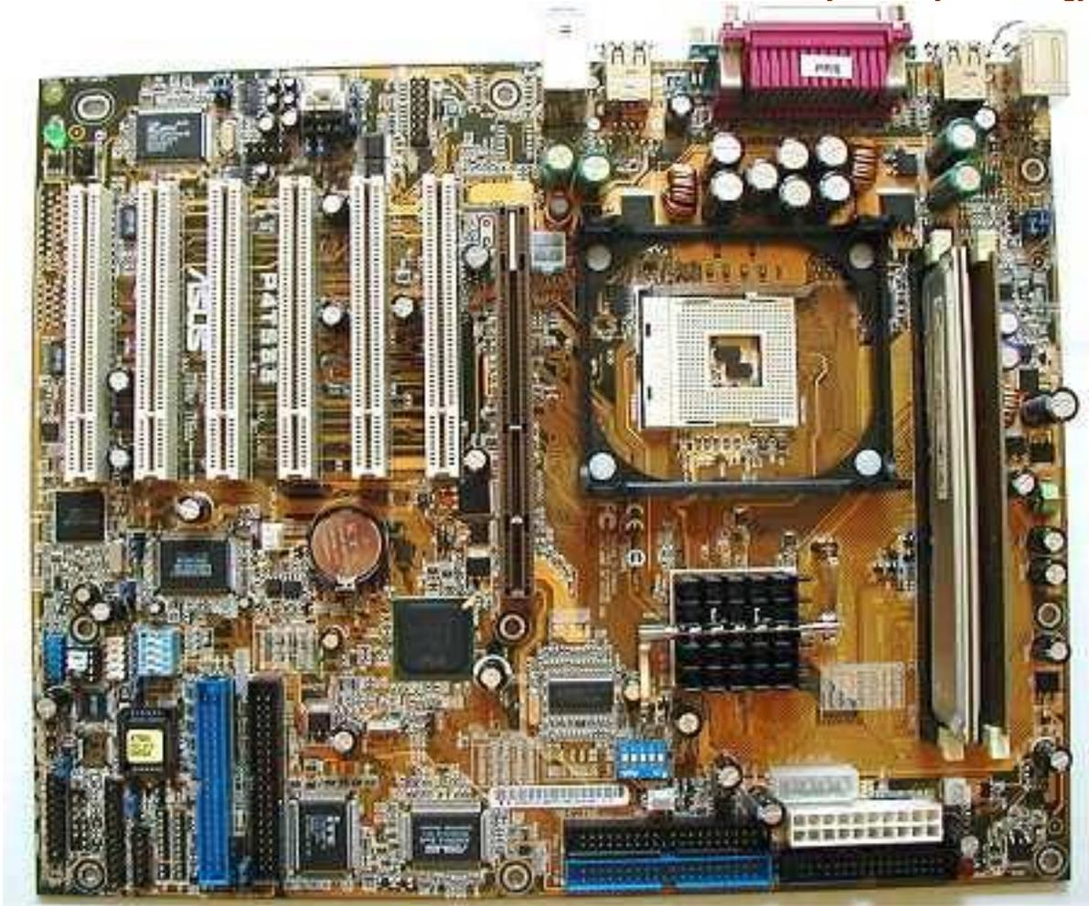
Luckily, the RDRAM channels were not the problem. When we lowered the clock multiplier to 16, the system was able to run rock stable at 150 MHz Quad (600 MHz) and even 159 MHz Quad was able to boot in Windows.
