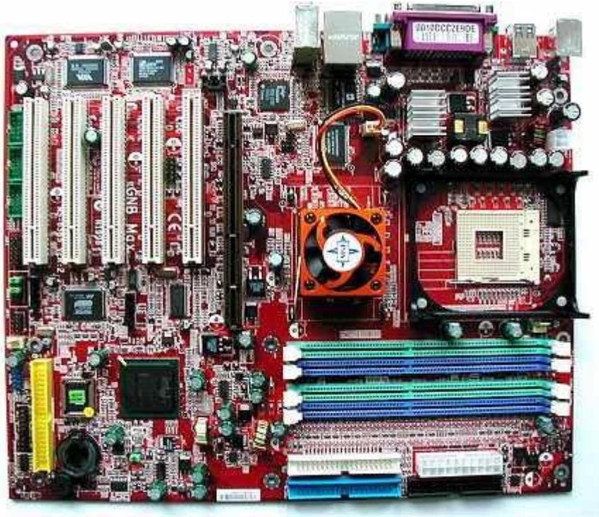
Although the board is equipped with the Promise PDC20376 RAID controller, RAID 0 or 1 will not be very fast on this board. The controller has only one IDE port, so you attach two IDE hard drives or 2 S-ATA drives, but not both at the same time. For RAID 0 harddisk setup however, it is best to put each harddisk on a different IDE port/channel to optimize performance.
