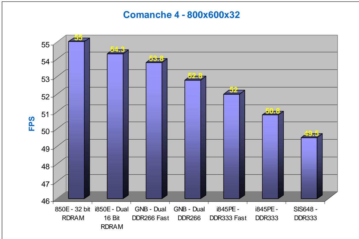
The Rambus board stays slightly ahead of the Granite Bay boards, even at 2-2-2-6.
