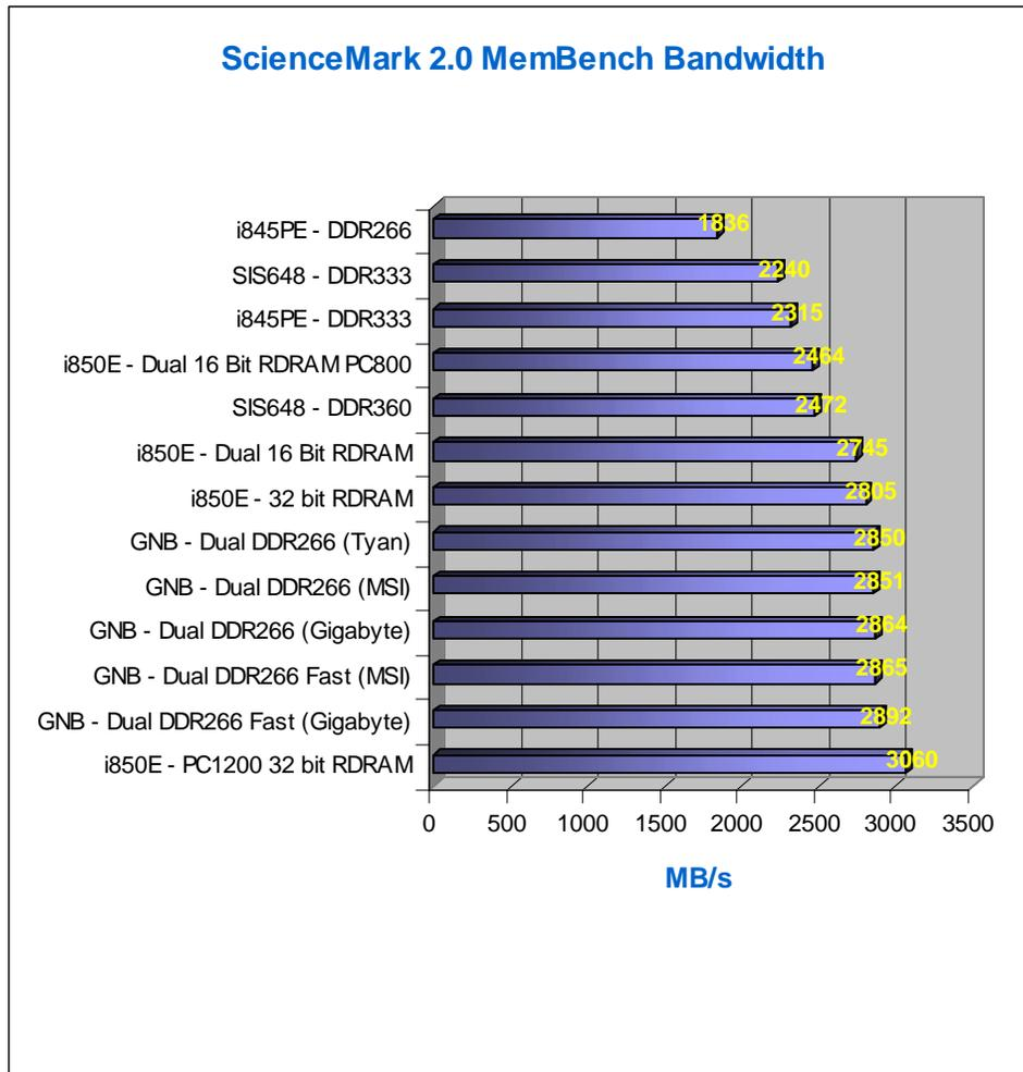
Interesting is that 32 bit RDRAM, which consists of two 16 bit channels on the RIMM, offers a little more bandwidth and slightly better latency than combining two channels of 16 bit RDRAM on a motherboard. Apparently, combing the two channels on a RIMM somewhat shortens the Rambus Transmission line and thus lowers the latency. This results in a small increase of the effective bandwidth.
