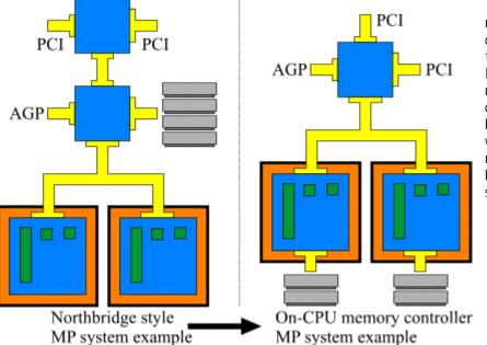
Multi-processor systems for CPUs with on-die memory controllers still need high-speed cache coherency connections, and also a way to access "non local" memory - this is a bit like having a system with multiple northbridges. Such a coherency/non-local connection could be rather like a "front side bus" in current multi-processor systems, which would mean that non-local memory requests would have similar latency and bandwidth characteristics as current systems.
