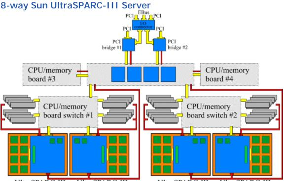
Chipset architecture: Sun's 8-way UltraSPARC-III workgroup servers (Sun Fire V880) use the same chipset on a CPU level as the 2way systems, though introduces some new features on a system level. Sun's entire UltraSPARC-III line is built upon the same basic chipset too. The system is split across 4 CPU/memory cards, each with 2 CPUs and up to 16GBytes of memory (currently), with each CPU controlling 8 DIMMs. The 4 CPU/memory
