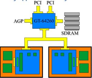
**Chipset architecture:** The basic architecture is similar to Intel's dual processor systems - two CPUs sharing a bus with an ASIC ("GT-64260") that has a memory controller. However, it seems the chipset Apple uses has the southbridge integrated as well, which should save costs, power, size and increase (I/O related) performance a little bit. Up to 1.5GByte/s of SDRAM is supported, though a newer chipset supports up to 2GByte/s of DDR SDRAM.
