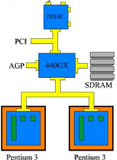
**Chipset architecture:** The main 2-way Pentium III chipset is the 440GX which uses normal SDRAM, though there is also the 840 chipset which uses two Rambus channels (like the 850 Pentium 4 chipset), both of which support up to 4GByte of main memory. The architecture is standard northbridge and southbridge, with the two Pentium IIIs sharing a single bus.
