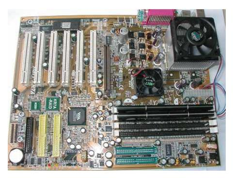
The board supports up to four 1 GB DIMMs for a total memory capacity of 4 GB, but only if you use registered (buffered) DDR modules. Registered modules carry a price premium, though at such module densities, it is not overly significant in our opinion. Crucial currently sells 512 MB PC2100 registered ECC modules for about \$15 more than the equivalent unbuffered, non-parity modules. When using strictly unbuffered modules, the KR7A-RAID is limited to 3 GB.
