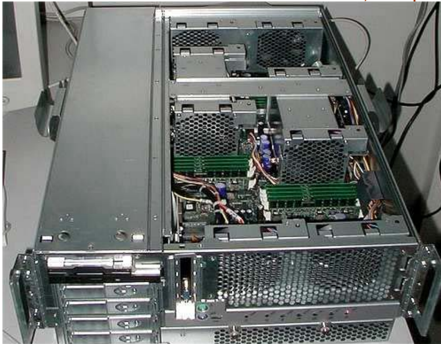
The Quartet server - A view of the four CPU nodes which are connected by 16/16-bit HT links
