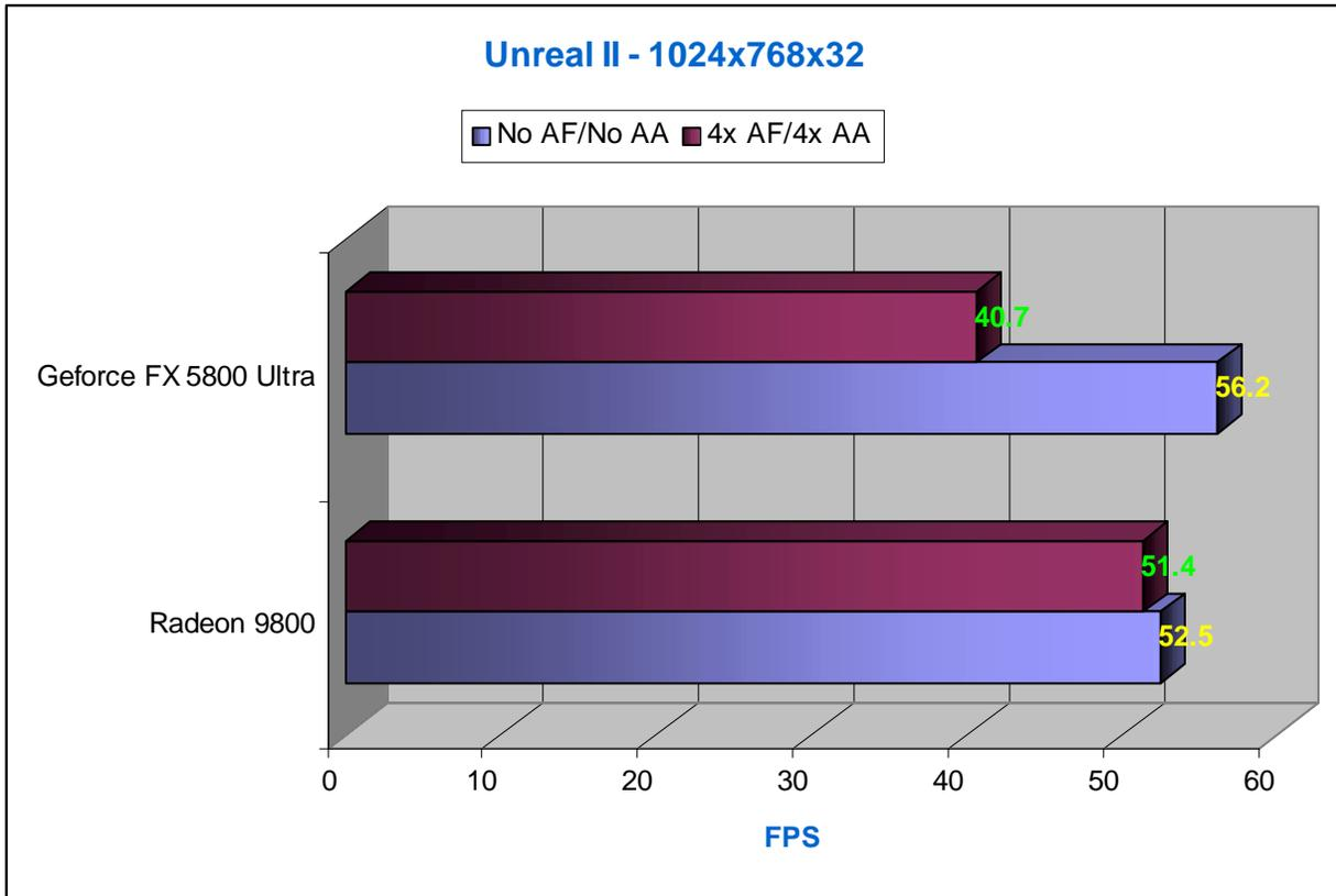
Unreal II presents another opportunity for the GeForce FX to take a slight lead, but again, only with both anisotropic filtering and anti-aliasing disabled. The performance impact associated with 4x AF and 4x AA on the GeForce FX is 28% in this test, while the drop on the Radeon 9800 Pro is practically within the margin of error.
