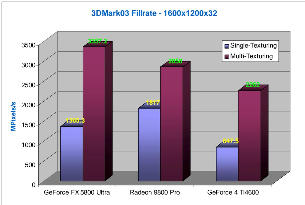
As you can clearly see from these results, the measured pixel fillrate of the GeForce FX (1365.3 MPixels/s) is well below the stated 4000 MPixels/s. It's also well below what the Radeon 9800 Pro achieves, despite the fact that the R350 core is rated with a lesser peak fillrate. In the case of multitexturing, however, the GeForce FX's fillrate is much closer to its theoretical peak.
