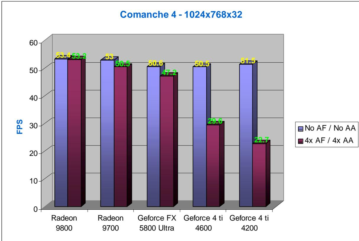
As a simulation, Comanche 4 is far more demanding on the CPU than what we saw previously with Unreal Tournament 2003. As a result, the framerates are much closer to each other, with only the GeForce 4 boards showing a significant decline in performance when 4x AF and 4x AA are enabled. 1024x768 is a bit low, however, so let's increase the resolution to 1280x1024:
