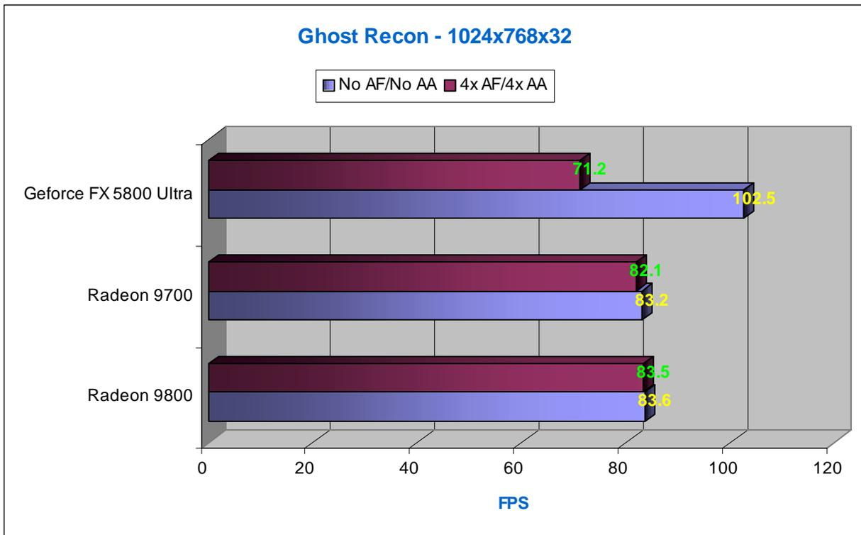
At last, the GeForce FX 5800 Ultra takes the lead, turning in a result that's 19% faster than the Radeon 9800 Pro with both anisotropic filtering and anti-aliasing disabled. Of course, the second mode -- 4x AF and 4x AA -- is far more likely to be the most common of the two (especially at 1024x768), and there the GeForce FX falls behind by about 15%.
