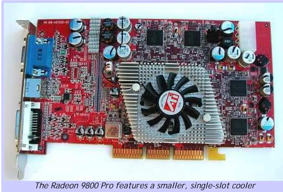
As you can see in the picture above, the Radeon 9800 Pro has a noticeably smaller heatsink and fan that fits within a single slot. Subjectively speaking, it is quieter than the GeForce FX and some Radeon 9700 Pro boards. The 128 MB Radeon 9800 Pro lists at US\$399.00 from ATI.
