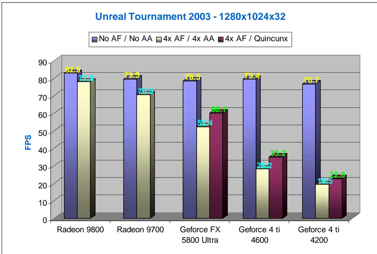
In this graph, anisotropic filtering and anti-aliasing are denoted by "AF" and "AA," respectively.
