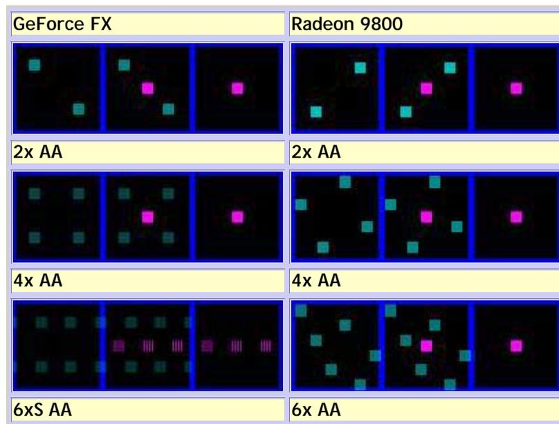
Looking at this comparison, the differences between implementations emerge quickly. Both the GeForce FX and Radeon 9800 use a rotated grid for 2x FSAA. In the case of 4x AA, however, the GeForce FX uses an ordered grid, as opposed to the rotated one used by the Radeon 9800.
