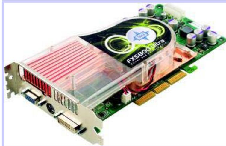
*The GeForce FX 5800 Ultra and its large two-slot cooler*
