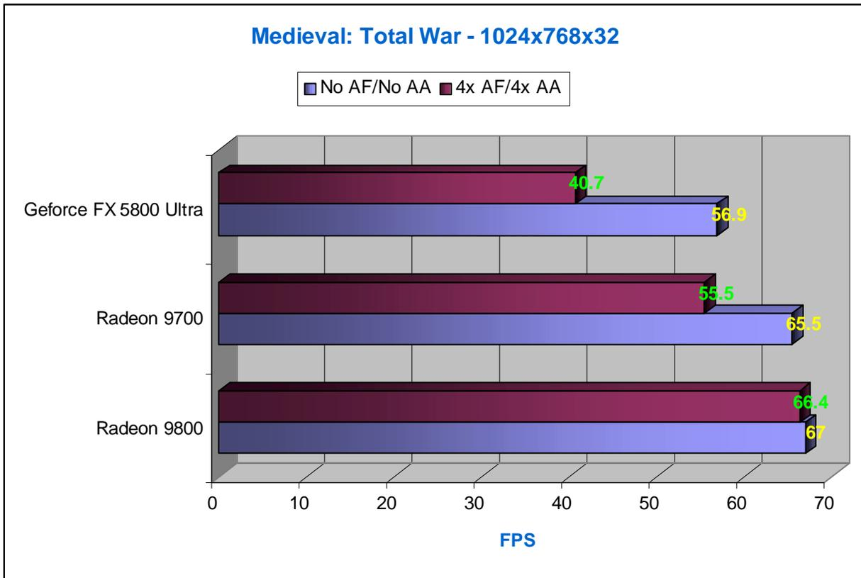
As mentioned above, this is a very CPU intensive game, and as such even the highest frame rates fall under the default refresh rate of most monitors at this resolution. Despite leading in NeverWinter Nights and Ghost Recon, we find that the GeForce FX 5800 Ultra is falling behind in Medieval: Total War. The difference is about 10 FPS with AF and AA disabled, but with 4x AF and 4x AA, the GeForce FX trails the leader by 39%.
