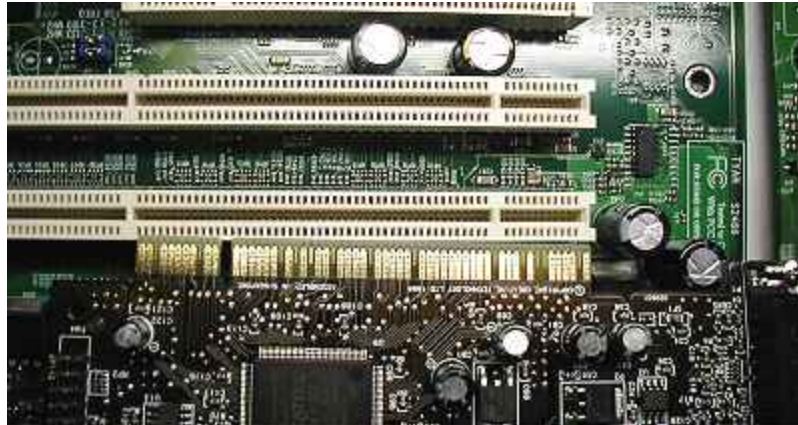
32-bit/33 MHz card in 64-bit/33 MHz slot: not possible
