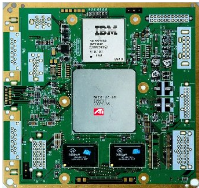
Gamecube System Board - Gekko (top), Flipper (center), Splash (bottom) Courtesy this Hotchips presentation by Peter Sandon
