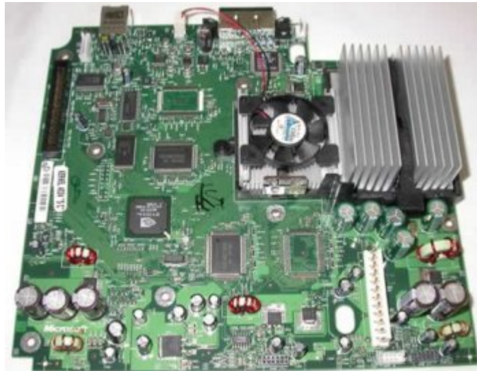
Xbox System Board - Pentium III/Celeron CPU (far-right, under heatsink), NV2A GPU (left of CPU, small heatsink /w fan)
