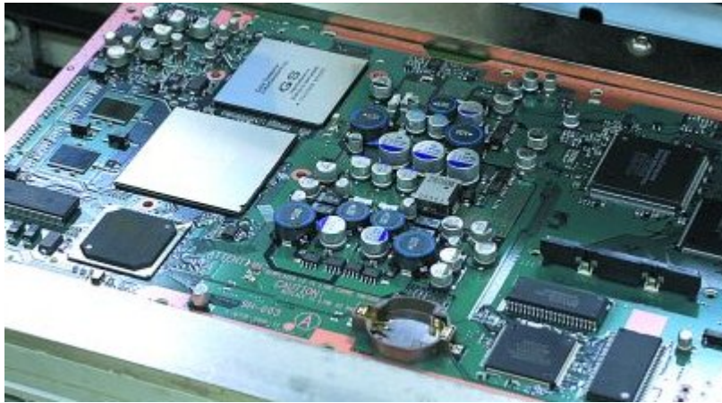
Playstation 2 System Board - Graphics Synthesizer (labeled), Emotion Engine (below/left of GS) Courtesy this article
